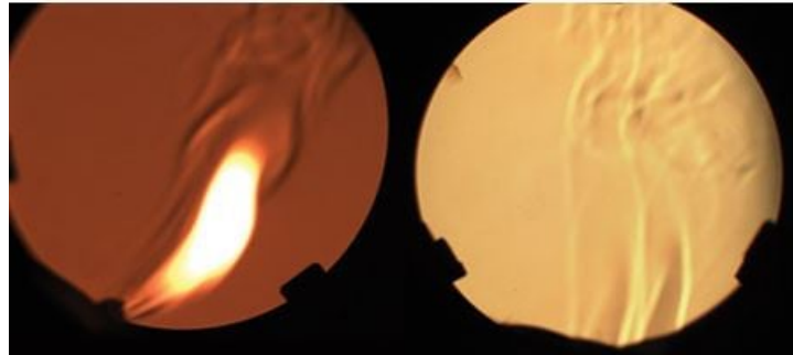
Flame Analysis using 6" Schlieren System
